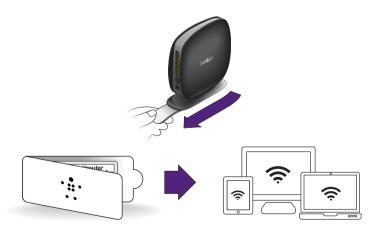
Type http://router to finish setup or try http://192.168.2.1
